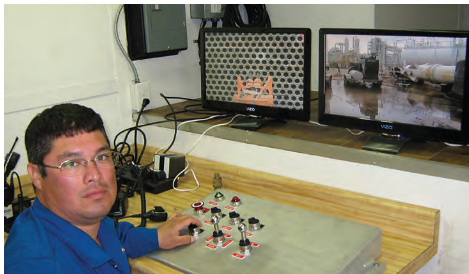
A VES employee operating remote hydro blasting technology at the Dow Freeport, Texas, facility.
