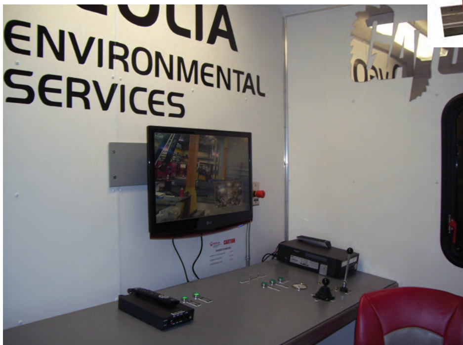
Enclosed trailer for viewing the inside of a tank cleaning job with the remotely operated Gator.
